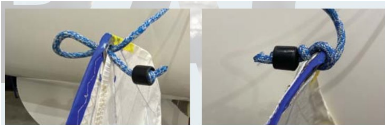
Marking the spinnaker sheet: a ball behind a knot at the thin end, looped through the clew ring
