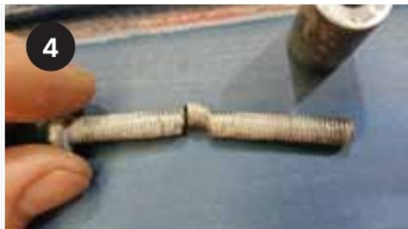
Picture 4: check the mast-step pin for signs of weakness
