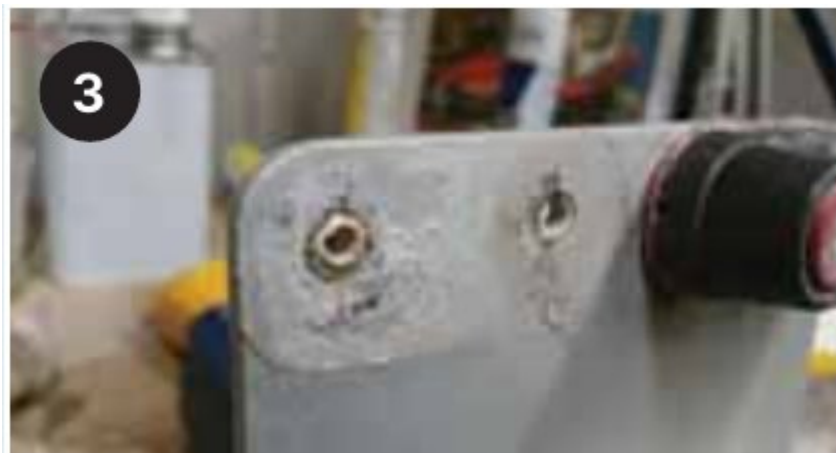
Picture 3: salt collecting between a cleat and its aluminium plate
