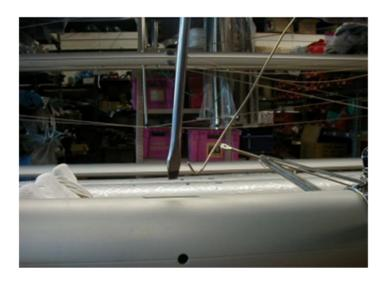
5. Pull all the wire through until the top swage is in the tube and can go no further
