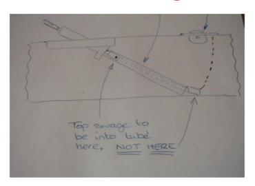
6. Pull the wire tight across the mast and mark from top of mast collar 272 mm and cut
