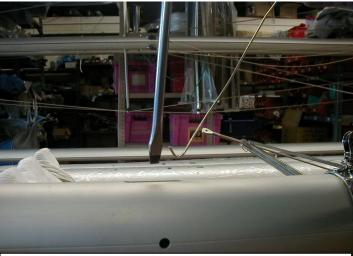
4. It is usefull to have a piece of wire with a hook to guide the forestay into the tube.
