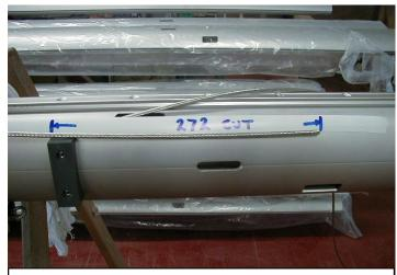
6. Pull the wire tight across the mast and mnark from top of mast collar 272 mm and cut.
