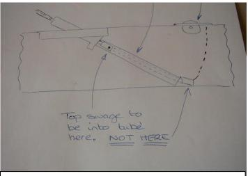
5. Pull all the wire through until the top swage is in the tube and can go no further.
