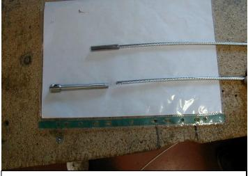
1. One end is swaged on, the other swage with the hole is loose.
