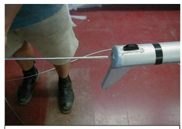
2. Put wire through hole in the mast.
