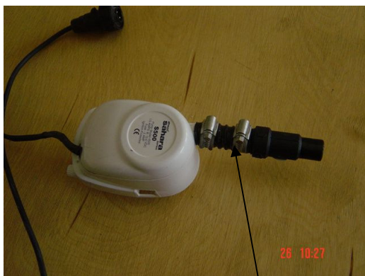
Undo hose clamp and flush through water in the direction of flow.
